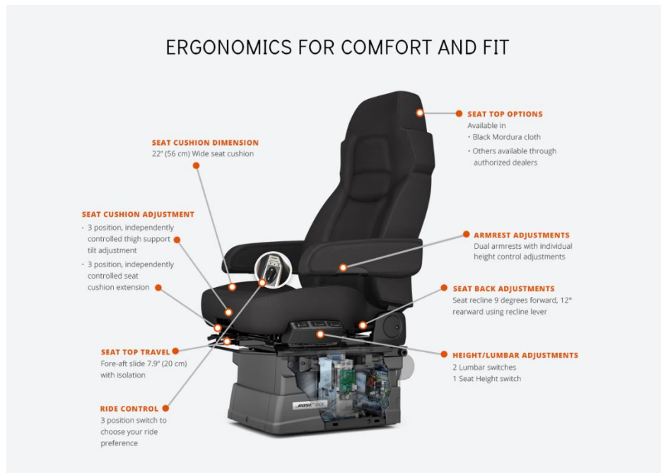
Figure 19: BOSE RIDE Truck seat with active vibration cancelling [33]
