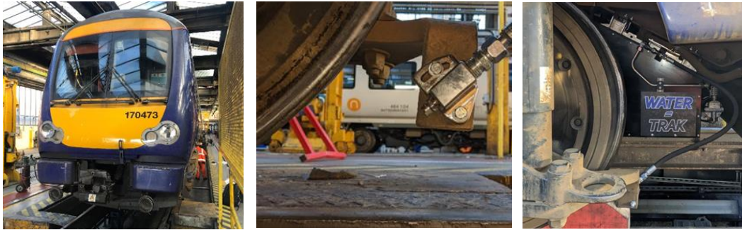
Figure 2: Water-Trak installed in Class 170
